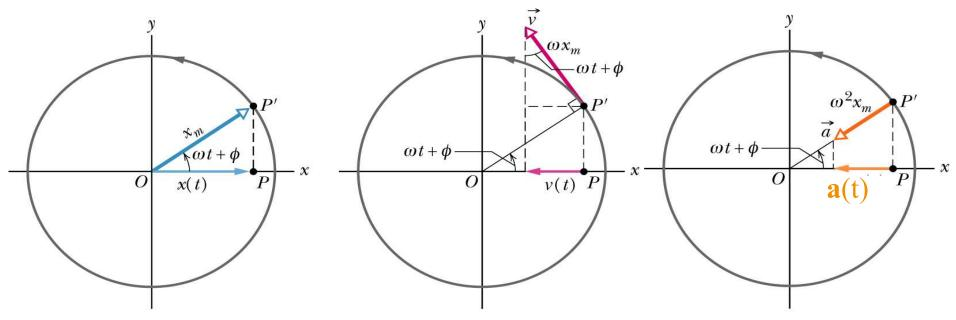
$$x(t) = x_{m} \cos(\omega t + \phi) \qquad v(t) = -\omega x_{m} \sin(\omega t + \phi) \qquad a(t) = -\omega^{2} x_{m} \cos(\omega t + \phi)$$
