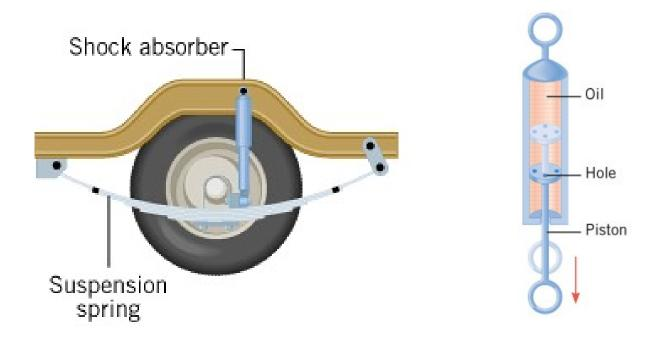
Typical automobile shock absorbers are designed to produce slightly under-damped motion
